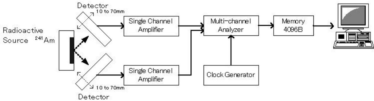
Fig. 1. Schematic diagram of random number generator.
